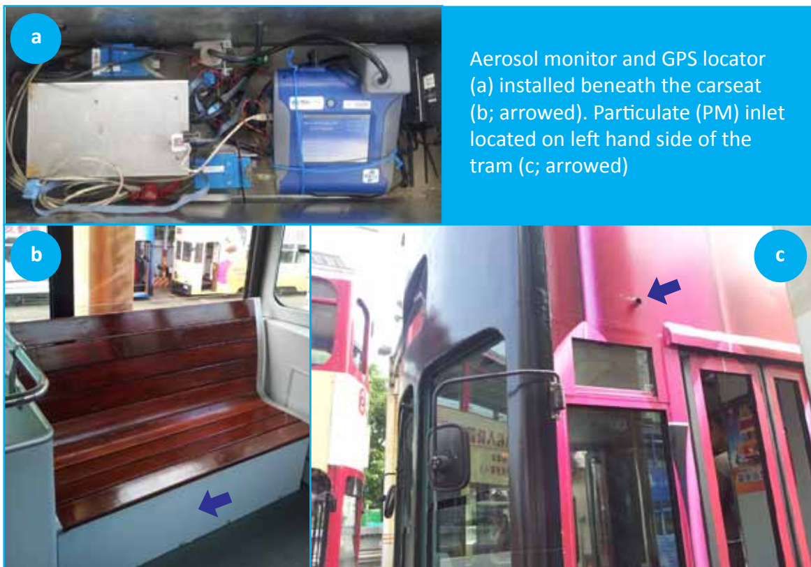
Figure 1. Air quality monitoring unit on the tramcar
